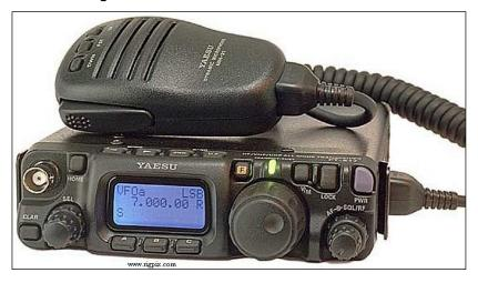
Some bigger stations use this as a driver, as the small RF power output, can reduce temperature drift associated with higher power transceivers in a small enclosure. The higher heat dissipation can also affect the longevity/reliability of transceivers.
